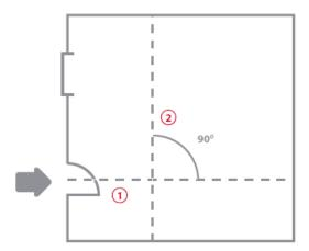
• Start spreading the glue on the subflooring at the intersection between the two axes.
